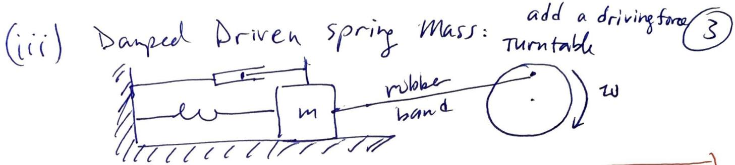
$$x'' + \left(\frac{b}{m}\right)x' + \left(\frac{k}{m}\right)x = A \cos(\omega t + \phi)$$
