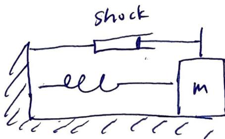
$$\begin{cases} F_{sp} = -kx \\ F_{drag} = -bv \\ -kx - bv = ma \end{cases} \quad \begin{matrix} \text{Newton's} \\ \text{Law} \end{matrix}$$
