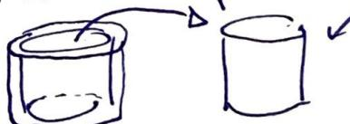
$$\begin{aligned}&= (35 \times 10^6 / ^\circ\text{C})(70 \text{ l})(40^\circ\text{C} - 20^\circ\text{C}) \\ &= \underline{0.049 \text{ l expansion}}\end{aligned}$$
