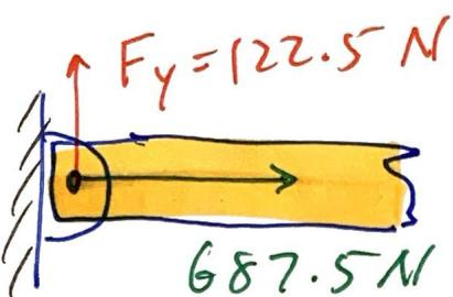
Pin keeps beam from sliding down wall
