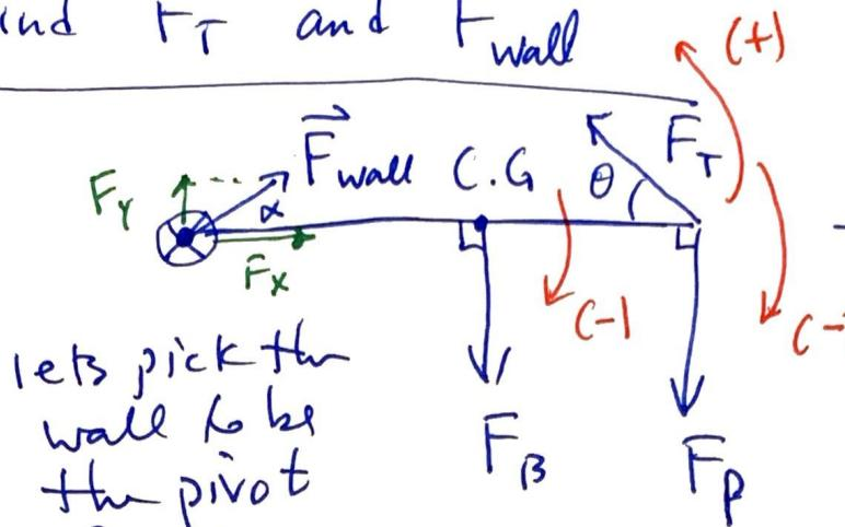
lets pick the wall to be the pivot for the torque eqn.
