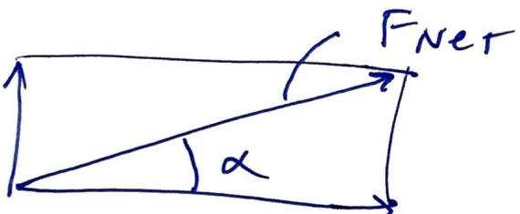
$$\left\{ \begin{array}{l} F_{net} = \sqrt{(687.5)^2 + (122.5)^2} \\ = 698.3 \text{ N} \\ \alpha = \tan^{-1} \left( \frac{122.5}{687.5} \right) \\ = \underline{\underline{10.10^\circ}} \end{array} \right.$$
