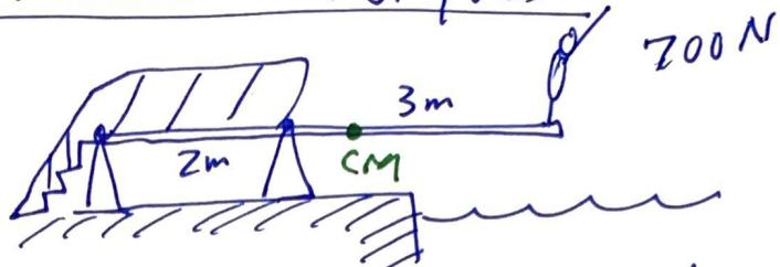
Q: Find the Forces on the two pylons supporting the board.
